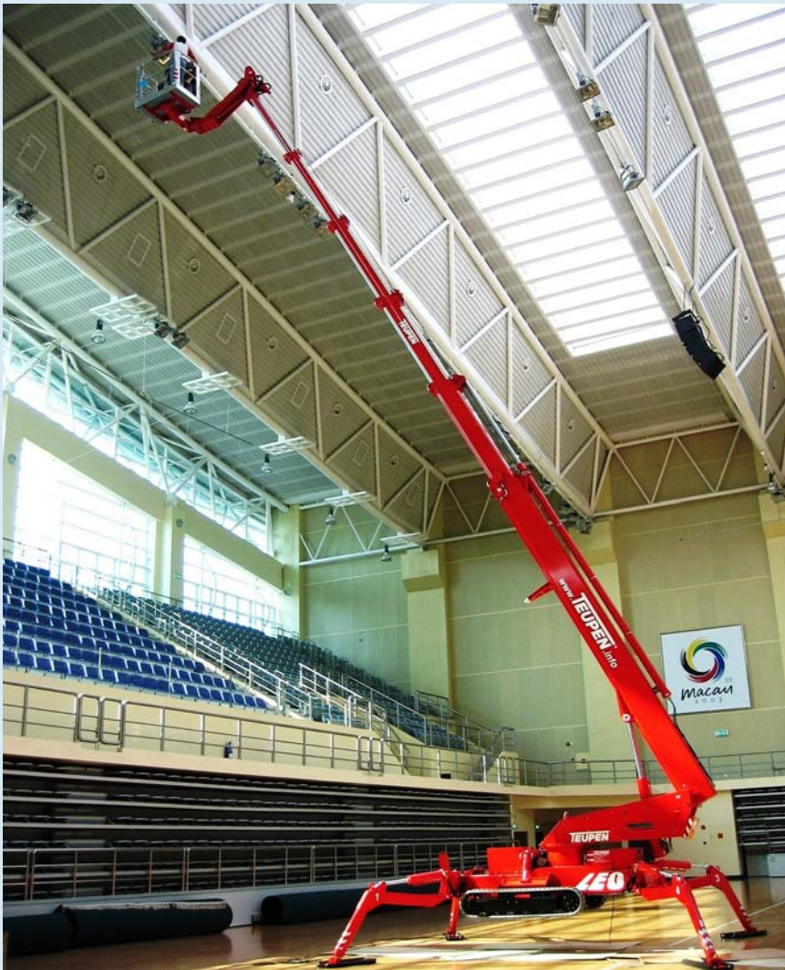
On the powerful track drive the LEO36T can be manoeuvred precisely. It even allows the machine climb steep slopes and stairs.
