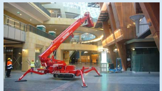
The automatic outrigger system levels out height differences perfectly. Additionally, two different outrigger setup positions are available.
