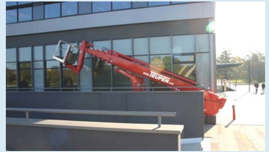
On the powerful track drive the LEO36T can be manoeuvred precisely. It even allows the machine climb steep slopes and stairs.
